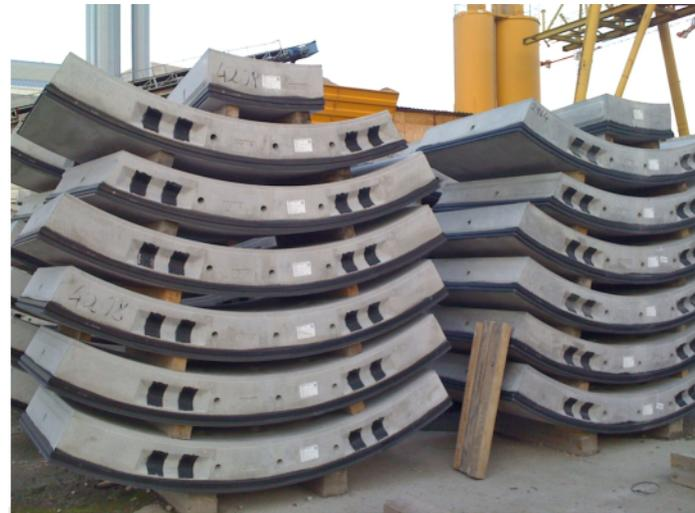
In case of special requirements concerning chemical resistance when used in extremely contaminated ground CTS offers alternative materials ( e.g. CR/SBR elastomer for better resistance against hydrocarbons found in ground water ). This alternative material can be offered as a reasonable compromise, but always under consideration of lowering the typical and physical properties of an EPDM-Compound with regard to aging performance and longevity.
